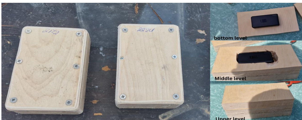
Figure 20. Construction of buoys with GPS with rectangular shape (Source: MCG)
