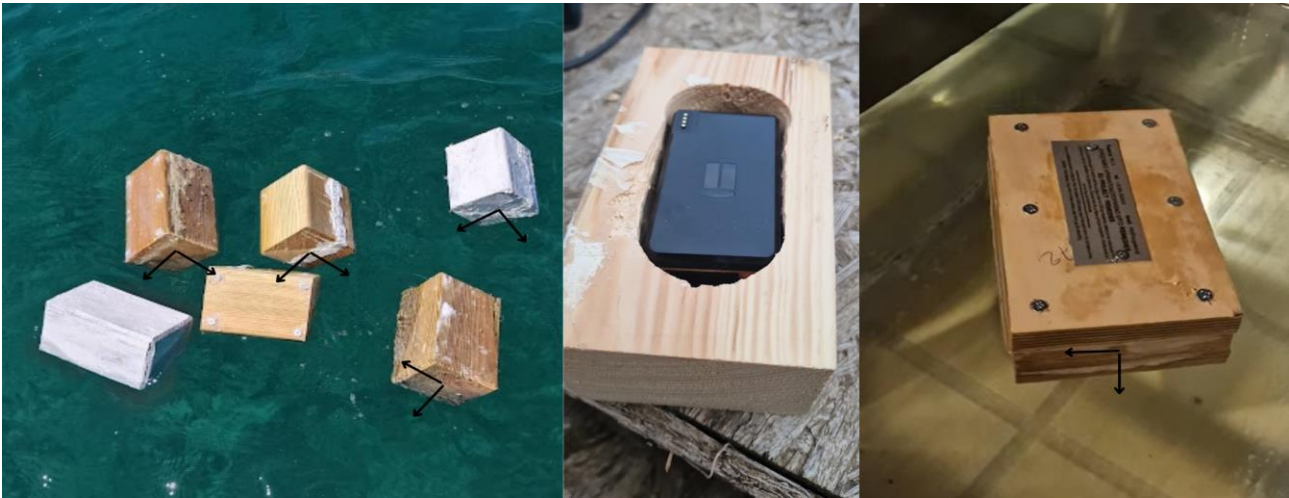
Figure 21. Buoys with GPS first test into water (Source: MCG).
