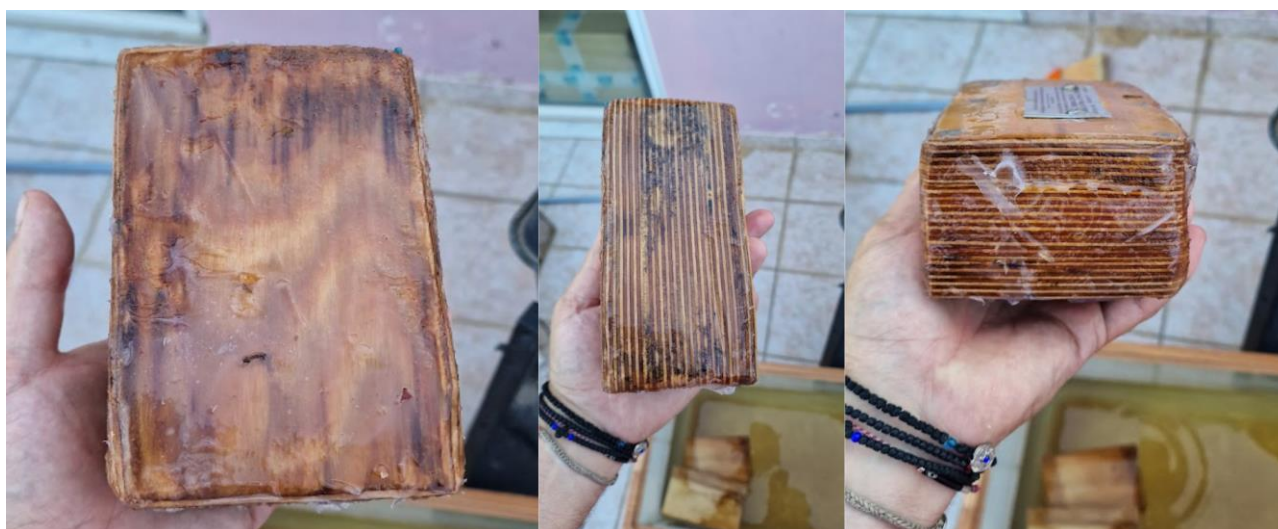
Figure 27. Damages and Degradations to Wooden Buoy During Testing (Source: MCG).
