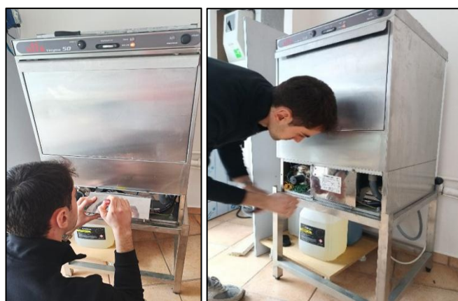
Figure 25 Dishwashing temperatures calibration
