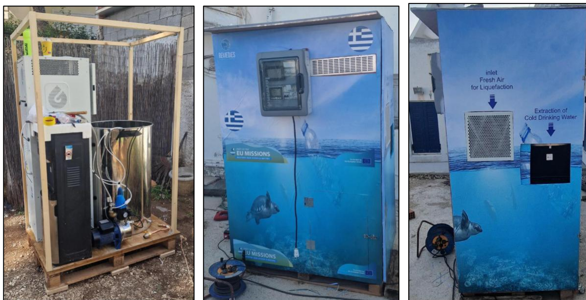
Figure 83 Installation of components (left) and complete AWG back side (middle) and front (right)
