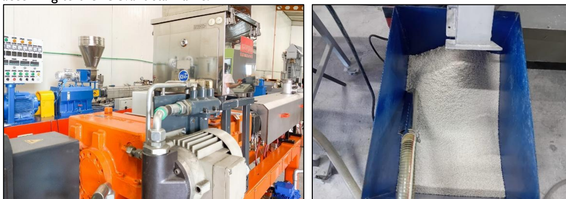
Figure 14 Compounding process at TRL7 (left) and drying (right)
