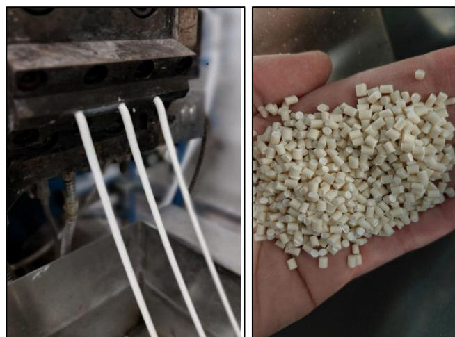
Figure 19 Compounding process of Remedies 6 on a twin screw extruder
