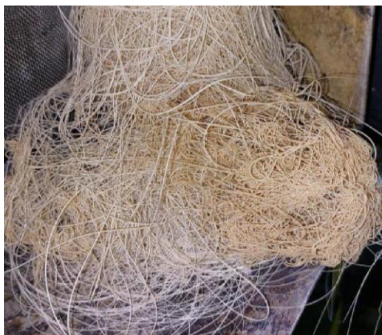
Figure 12 - Representation of the degradation that occurs at low extrusion speeds for compound 12. Starch/PBAT:PHA.
