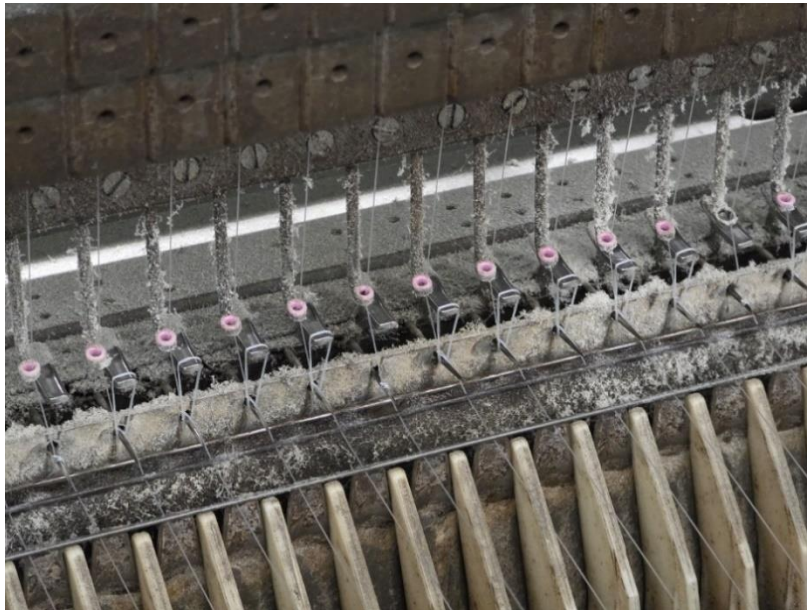
Figure 73 - Needlebed with the “dust” on the knitting elements
