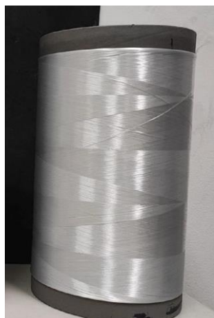
Figure 9 - Example of multifilament bobbin of "9" Fibre 5.
