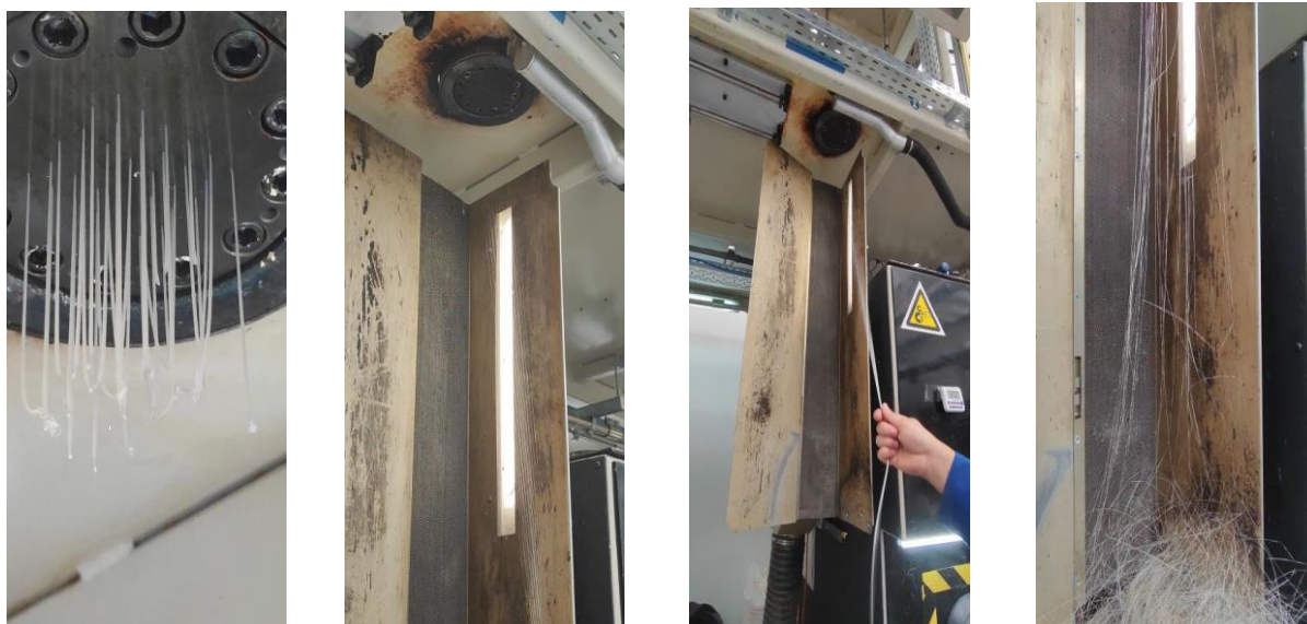
Figure 32 - Spinning trials: a) Low extrusion temperatures (B_T1), Low throughput; b) Low extrusion temperatures (B_T1), High throughput; c) High extrusion temperatures (B_T2), Low throughput; d) High extrusion temperatures (B_T2), High throughput.
