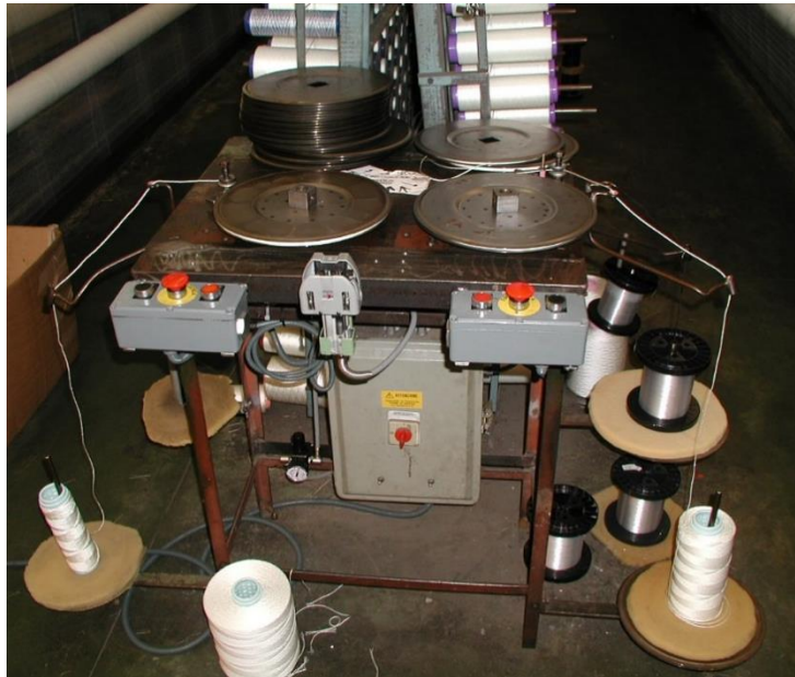
Figure 70 - The manual spool winder used to fill the spools
