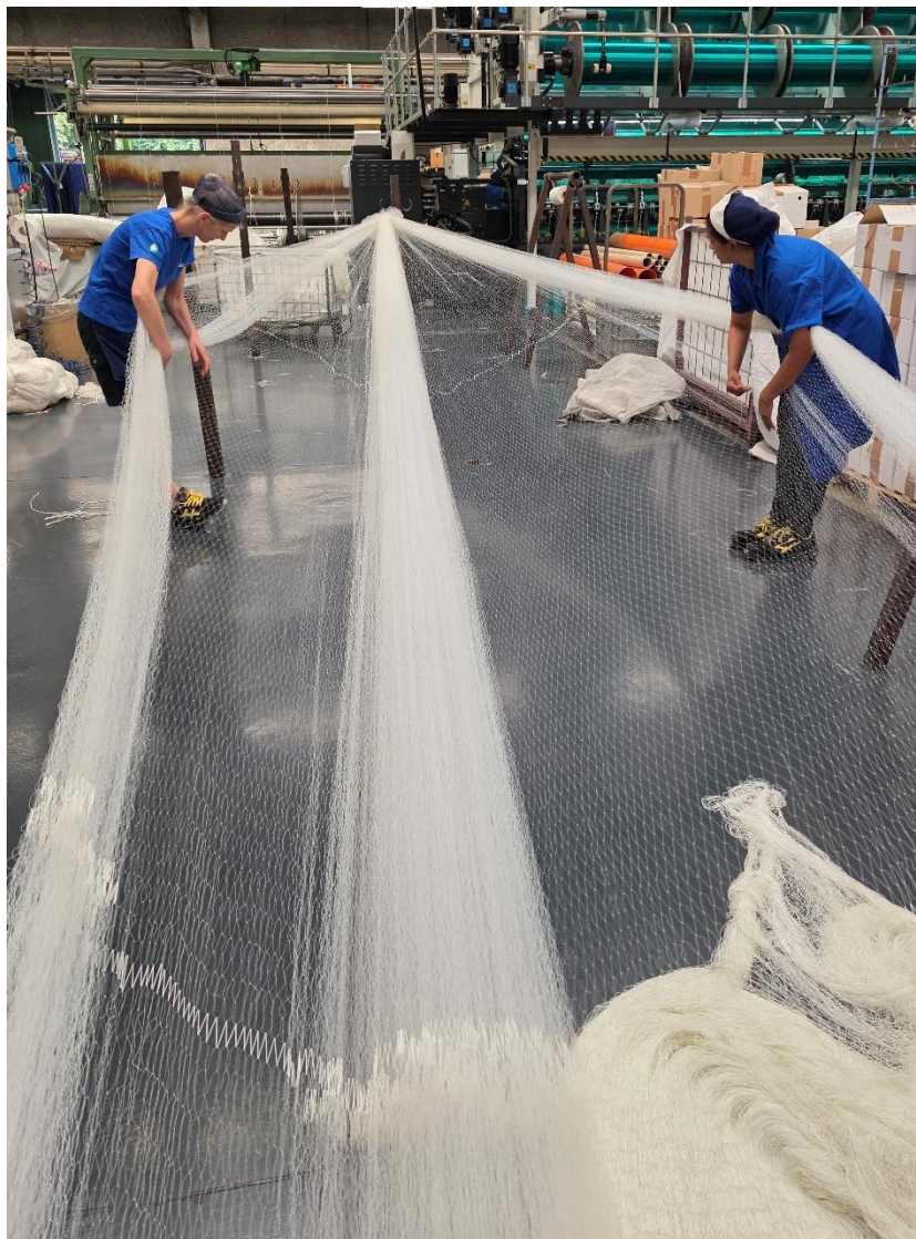
Figure 75 - Two operators inspect each part of the opened net
