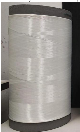
Figure 10 - Example of multifilament bobbin of "11" Fibre 4.
