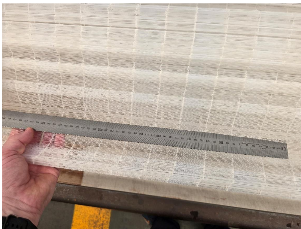
Figure 79 - The net stretched is measured to reach the correct mesh size
