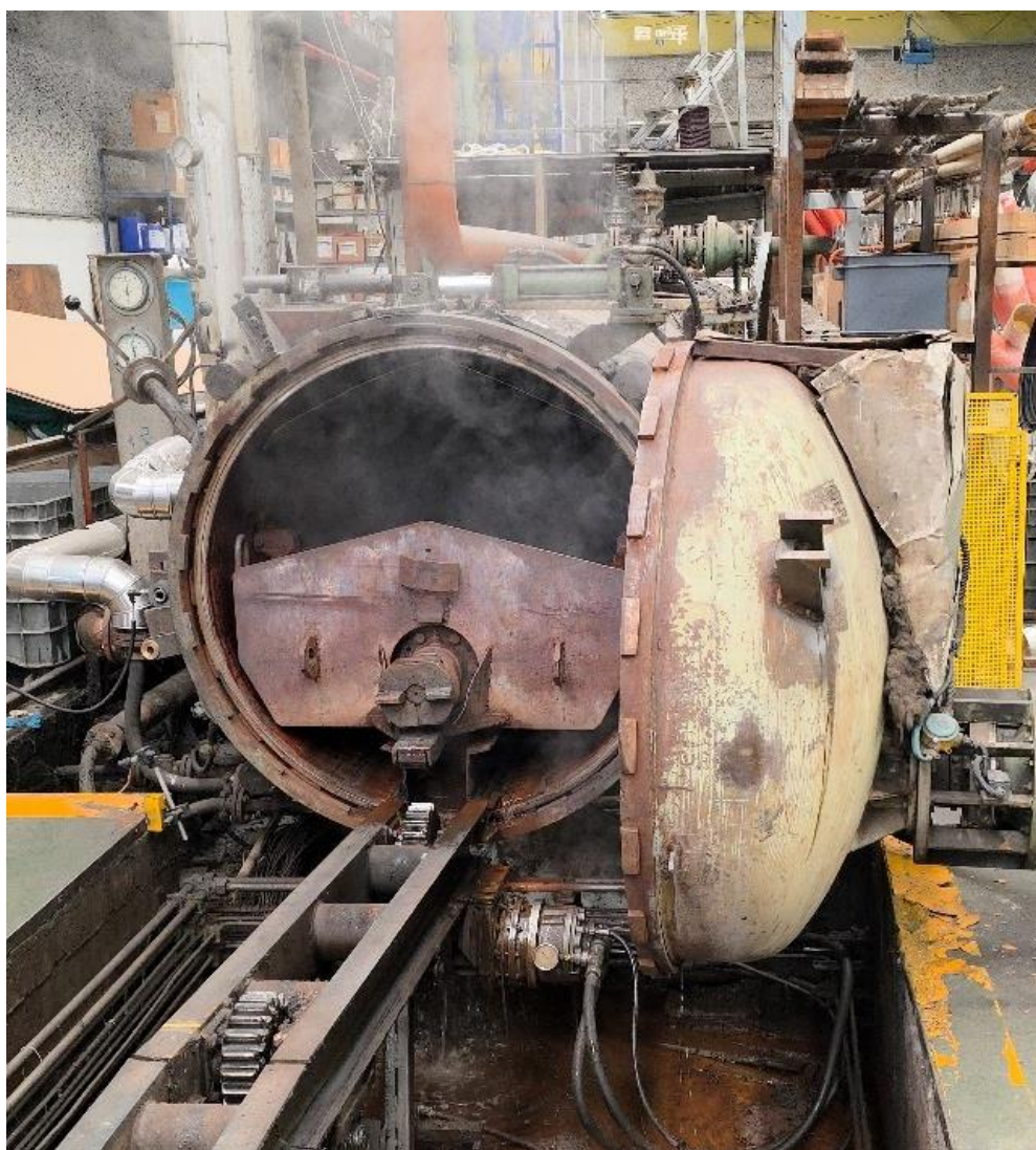
Figure 80 - The opening of the vacuum autoclave after steam heat setting treatment
