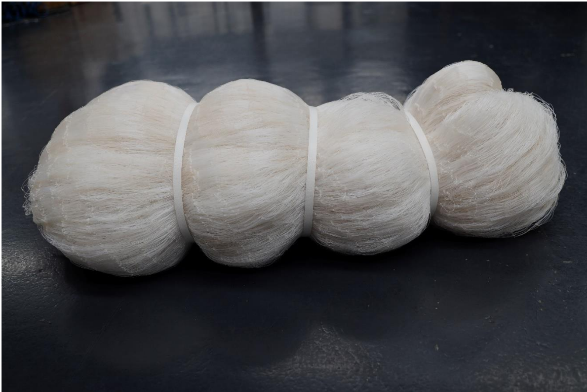
Figure 82 - The final appearance of a bale of knotted bio-degradable monofilament net
