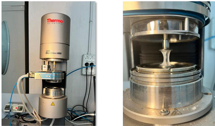
Figure 3 - Rotational rheometer Thermo Scientific Haake RheoStress 6000.
