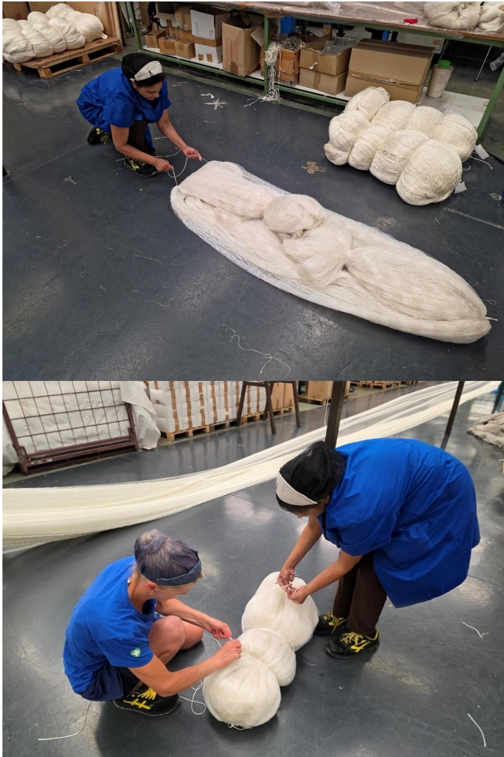
Figure 81 - The operators are packing the 4 nets in one small bale
