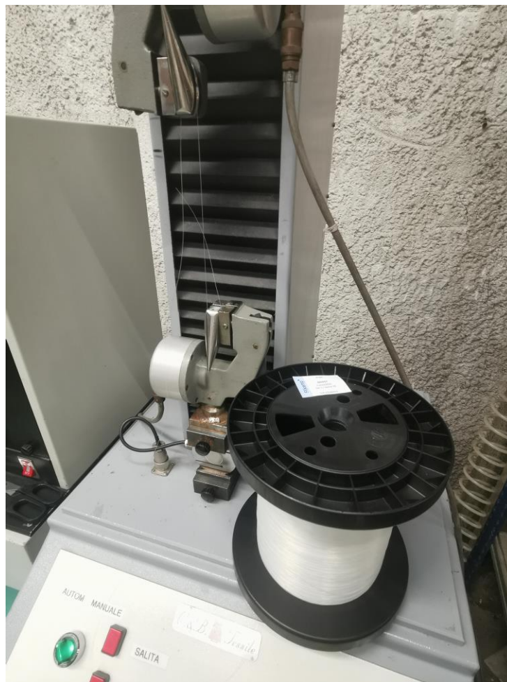
Figure 58 - The Dynamometer used to test the monofilament yarn
