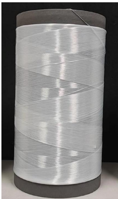
Figure 7 - Example of multifilament bobbin of "2" Fibre 1
