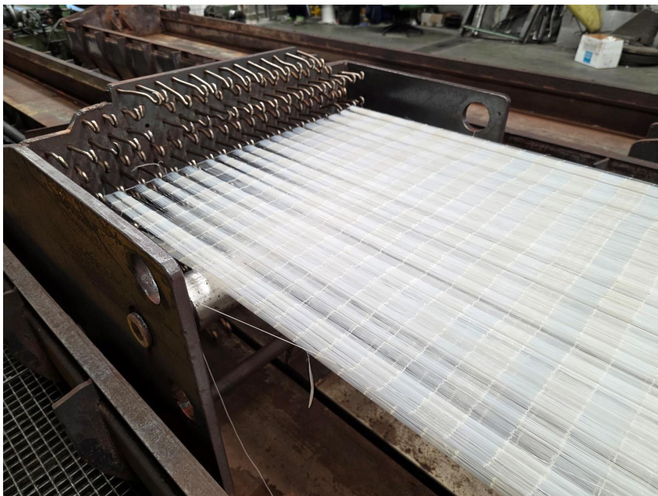
Figure 76 - One of the special ends where the iron combs are fixed
