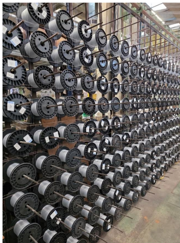
Figure 66 - The creel loaded with the 200 DIN bobbins
