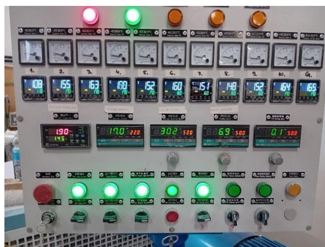
Figure 50 - Processing and control parameters during compounding step
