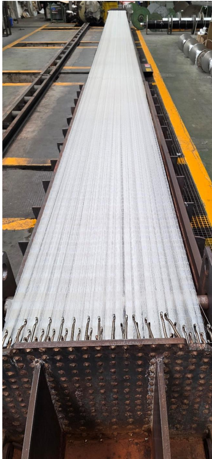
Figure 77 - The net loaded on the 25mt carrier of the heat setting machine
