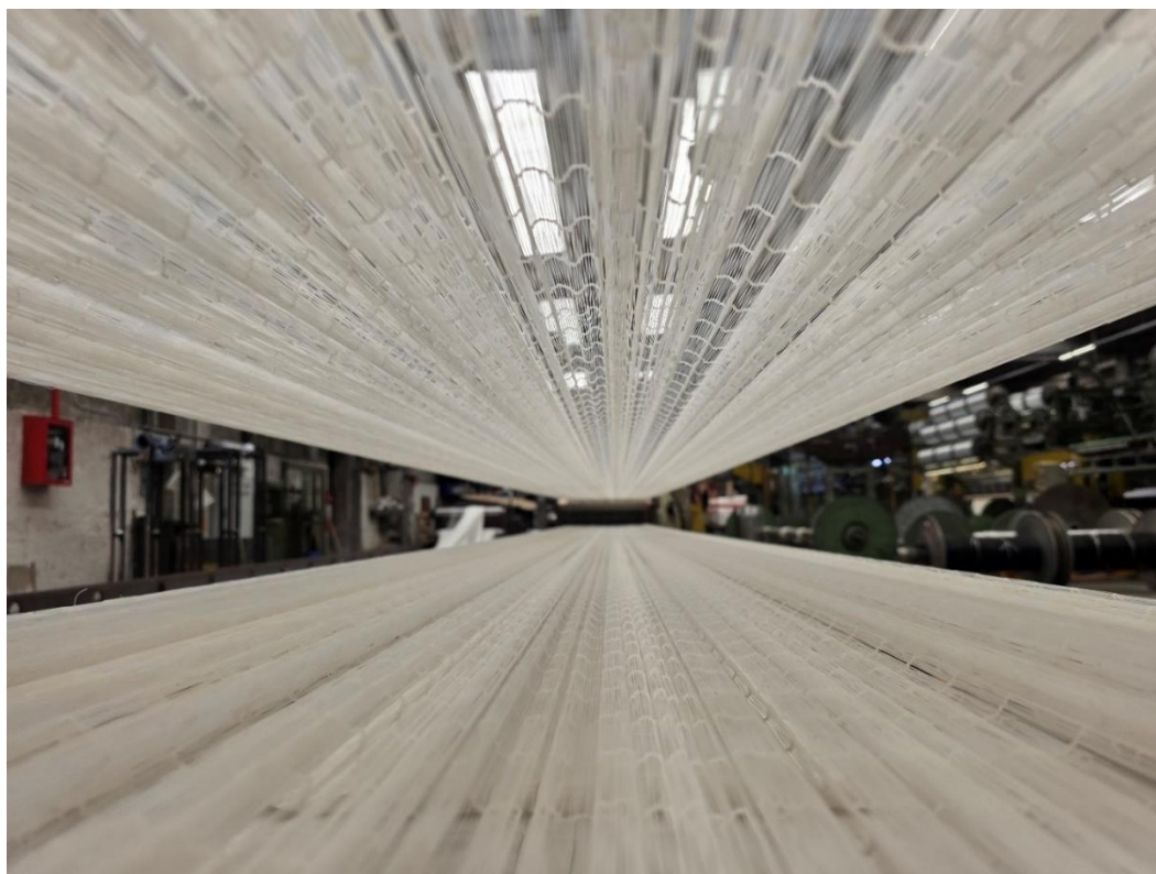
Figure 78 - A view of the 2 nets stretched on the carrier
