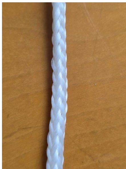
Figure 93 - The aspect of the braided rope made of bio-degradable monofilament
