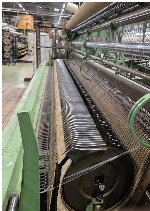
Figure 71 - Particular of the loom's carrier where are loaded the spools
