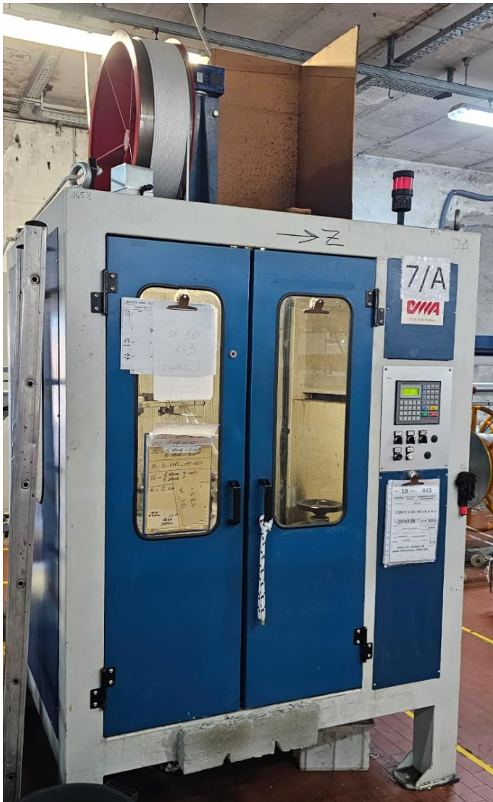
Figure 90 - Braiding machine with a detail view of the 12 rotating carriers
