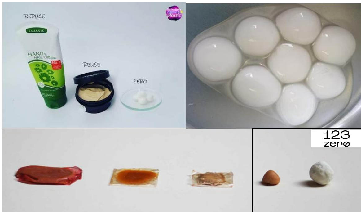
Figure 10: Visual representation of the evolution in the development of the seaweed zero-waste packaging's and coatings for creams and shampoo from the time of 2018-2020 and variation of the product without coating in the shape of the ball (Source: Scientists against plastic Instagram and 123zero).
