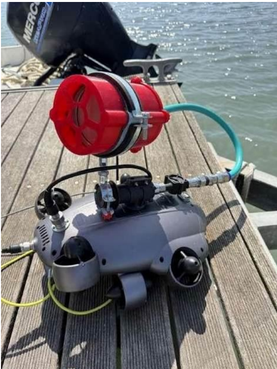
Underwater drone with the CLERA sampling module
